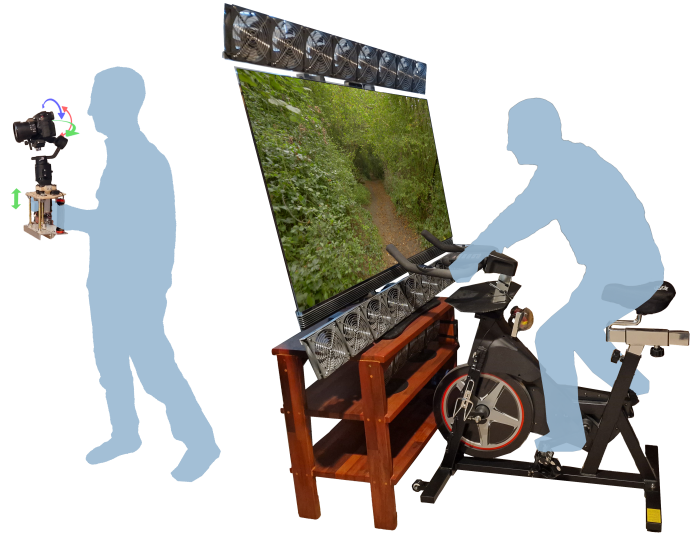
Figure 1: Hand-held video capture rig (left) and stationary cycling rig (right). A commodity 3-axis gimbal is augmented with a custom vertical stabilization system. The capture vantage point and field of view are matched to the 55” UHD display of the playback rig.
